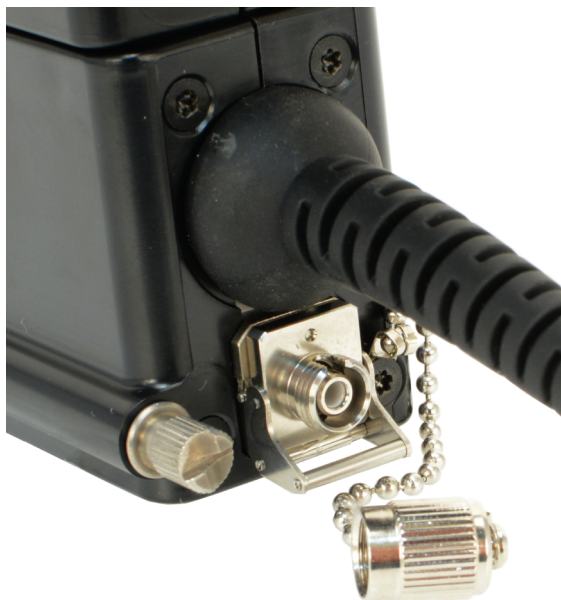
Figure 9: Removing the metal dust-cap from the optical connector
