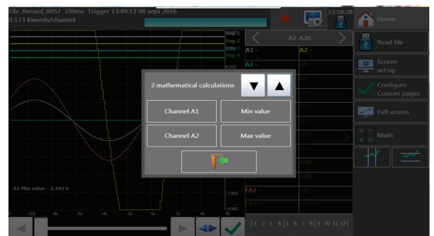
Math calculations between channels
