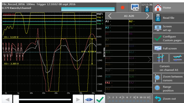
Measurement display with zoom and cursors
