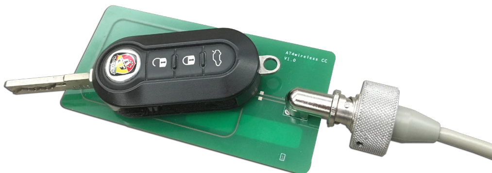
Figure 2. Sniffing out key fob RF signals.
